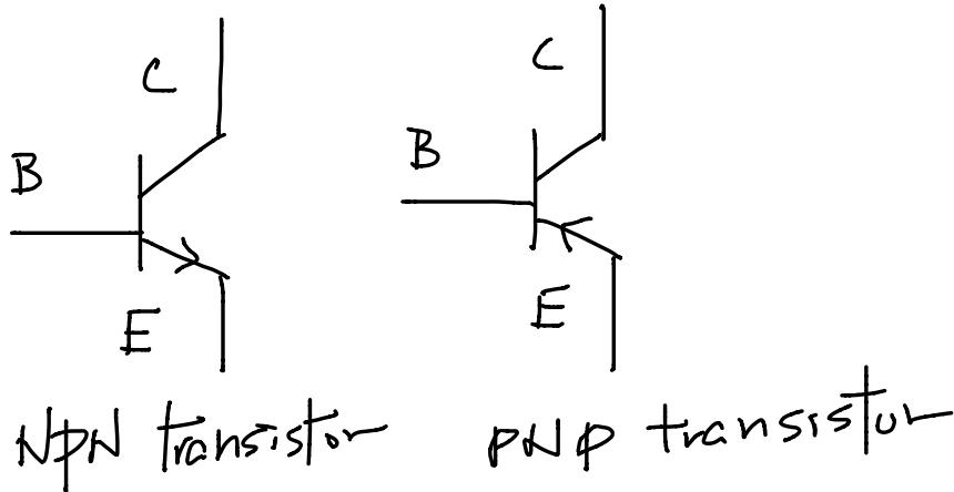
Transistor (transconductance resistor) is a three terminal device to switch or amplifier signals.
