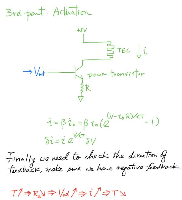
Al temp thermistor feedback actuator Al temp.
