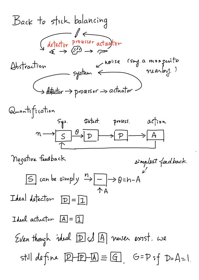
error signal & : deviation from our target (setpoint). n-D-G  $\theta = n - G\theta \Rightarrow \theta = \frac{n}{1 + G}$ Without feedback (G=0), we have Q=n. So noise is suppressed by (1+G). Thus to suppress the maise we just make G infinite. Poes that work? No, it will be imstable, some reason you fell when you learned biking for The 1st time. Solution to stablize an upside-down stick? Or temperature in a car? A concrete example: Temp serve you will work on: Air conditioning:
