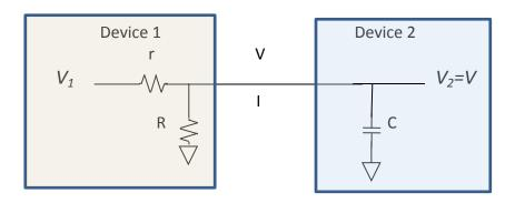
(B) Bandpass. Insert an *RLC* circuit between Device 1 and Device 2 such that only the signal at a desired angular frequency  $w_0$  can be delivered to Device 2 with 100% efficiency. Frequencies far from  $w_0$  will be suppressed.
