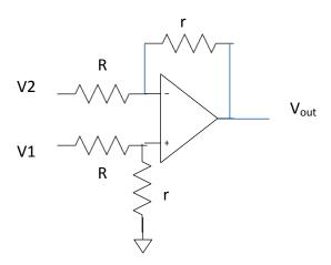
(B) Design an op-amp circuit to process two signals V1 and V2 such that  $V_{out}(t)=V_1(t)+2dV_2(t)/dt$ .
