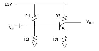
(c) Continue (B), derive  $V_{\text{out}}$  as a function of  $V_{\text{in}}$  when the amplification is working properly.
