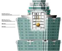
a) We model the building as a point mass  $m_1$  located at  $x_1(t)$ . It is connected to the wall with a spring with force constant  $k_1$ . Earthquake is modelled as the displacement of the wall by w(t). The motion of the building can be described as
