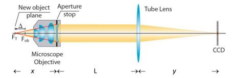
We consider an object on the left side of the microscope objective with the working distance of x, the distance between the object and the objective.) For simplicity, we assume the objective is a thin lens, and it collimates the light coming from the object onto the tube lens. The tube lens then forms an image on the CCD. Assume the objective has a focal length of  $f_1$  and the tube lens has a focal length of  $f_2$ .
