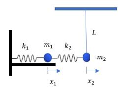
Point mass  $m_1$  on a frictionless horizontal plane is connected to a spring with force constant  $k_1$ . An ideal pendulum of length L with the bob of mass  $m_2$  (gravitational force is  $m_2g$ ) couples to  $m_1$  through a second spring with force constant  $k_2$ . In equilibrium their displacements are  $x_1=x_2=0$ . Here we consider small amplitude oscillations  $x_1,x_2\ll L$  away from equilibrium in the following cases
