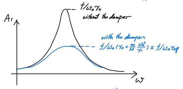
Effective new damping  $Y_{eff} = Y_0 + \frac{m}{M} \frac{\omega_0^2}{\gamma_1}$ Building shaking sup is reduced by a factor of  $(1 + \frac{m}{M} \frac{\omega_0^2}{\gamma_0 \gamma_1})$ .
