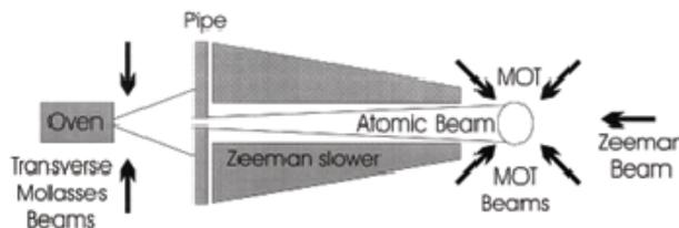
Here the atoms are ejected from the oven with a typical initial velocity of 300m/s, slowed by the Zeeman slower beam, and captured in a MOT. The Zeeman slower magnetic field is used to cancel the Doppler shift for atoms moving at high velocity.
