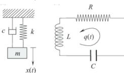
dissipates the energy and an external force F(t) can be applied to the mass.
