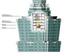
Let's figure out how it works. Vibration of the building with mass M due to external force F(t) can be modeled
